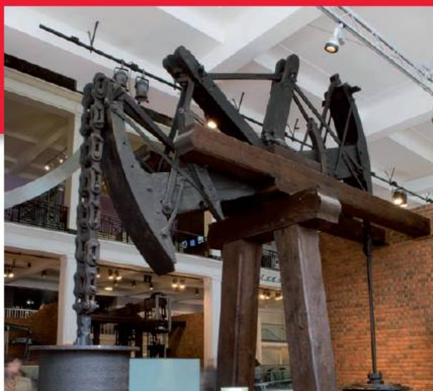
■ Figure 1.7 Old Bess is the oldest surviving Watt engine, and the third-oldest surviving beam engine. It is now housed and preserved in the Power Gallery of the Science Museum, London
