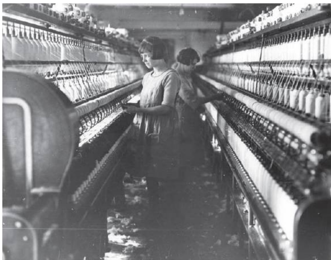
■ Figure 1.17 Ring spinners in a cotton factory in the north of England, c.1890
